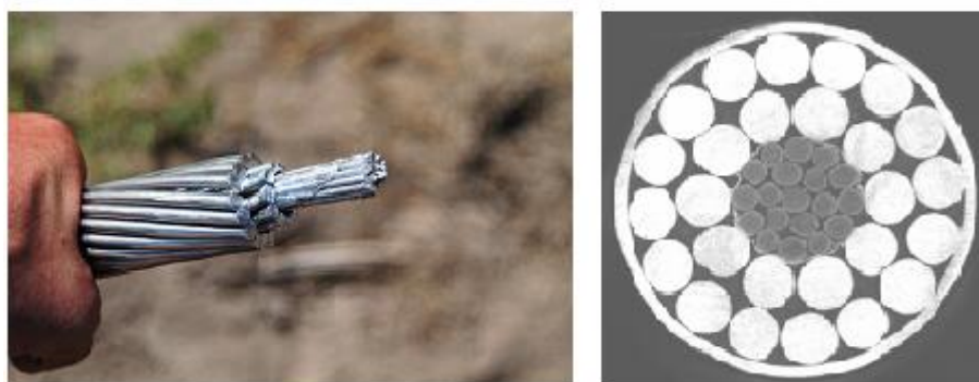
Figure 7-16 ACCR (3M) conductor and its cross-sectional area
