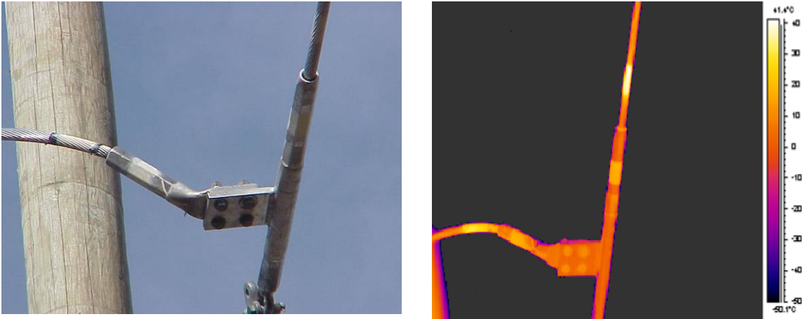
Figure 7-6 Visual and IR images of a dead-end assembly on a HTLS transmission system
