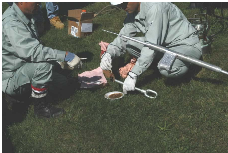
Figure 5-5 Application of high-temperature grease on core-grip portion
