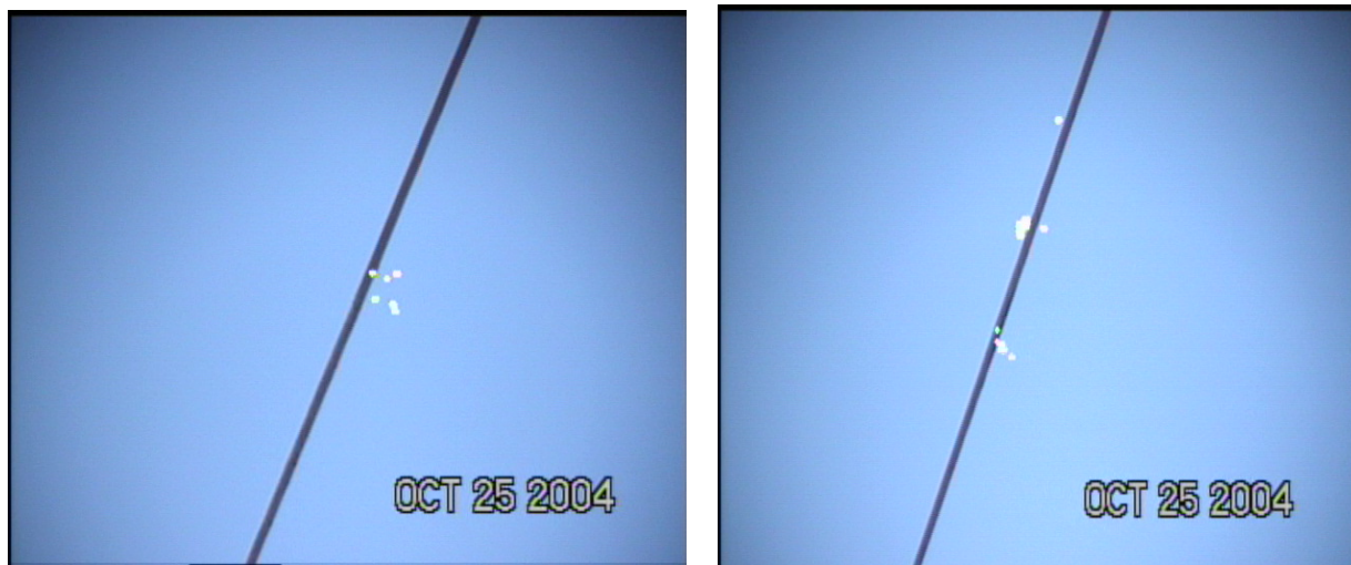
Figure 7-4 Corona observations on HTLS conductor surfaces installed in one of the field trial sites
