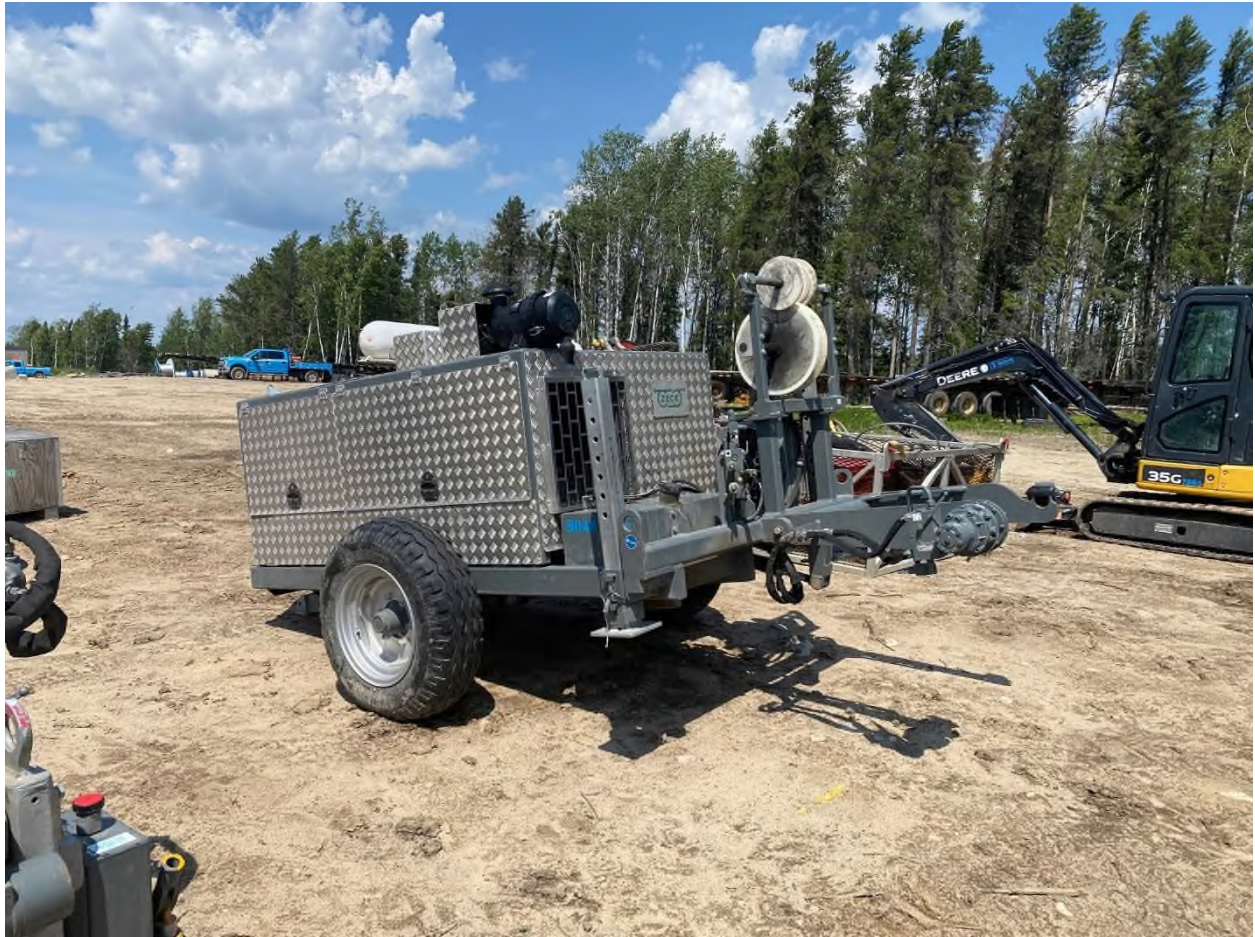
Photo 13: Heli-portable stringing gear
