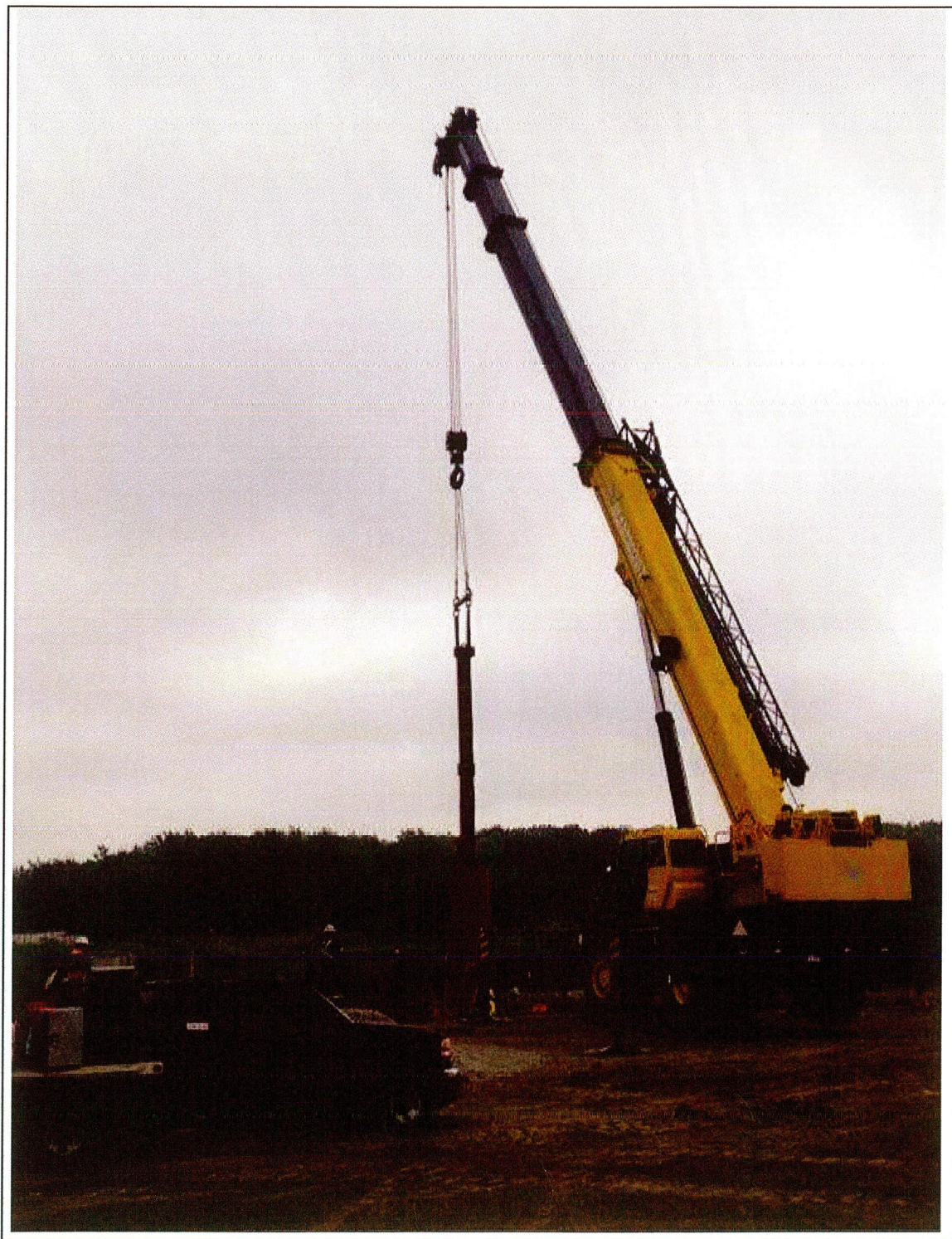
Figure 5: Typical Crane for Moving Fittings
