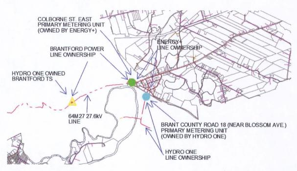
The source of the power is normally from an Energy+ owned three phase 27.6kV line on the Hydro One Networks owned Brantford TS 64M27 feeder. Brantford Power owns the 64M27 feeder from Brantford TS to the service area boundary with Energy+. At the service area boundary between Brantford Power and Energy+ on Colborne Street East, there is an Energy+ owned 27.6kV primary metering unit to measure the power withdrawn from Brantford Power's
