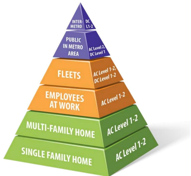
Figure 4: Charging Pyramid. Source: US DOE.
