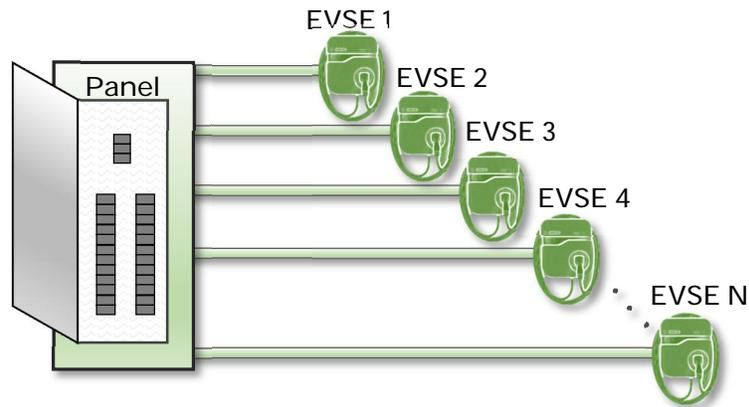
Figure 1: Dedicated circuit configuration of EVSE.
