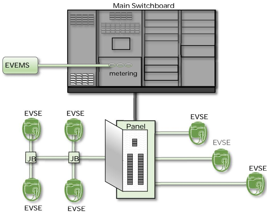
Figure 3: Service monitoring configuration of EVSE with EVEMS.
