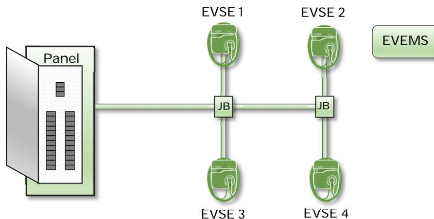
Figure 2: Load sharing configuration of EVSE with EVEMS.
