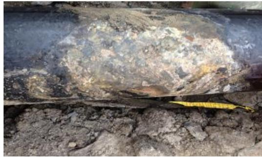
**Figure 5.2-54: Coating damages**
