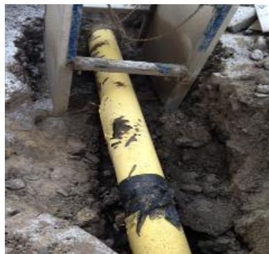
**Figure 5.2-53: Gouges and dents due to latent damages**
