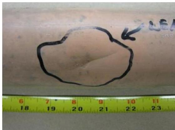
Figure 5.2-59: Sample of Aldyl-A Pipe with Crack Failure
