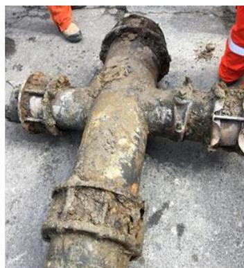
**Figure 5.2-23: Detail of fabricated fitting after removal**
