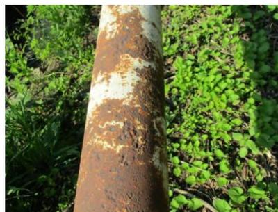
Figure 5.2-14: Coating degradation and corrosion pitting
