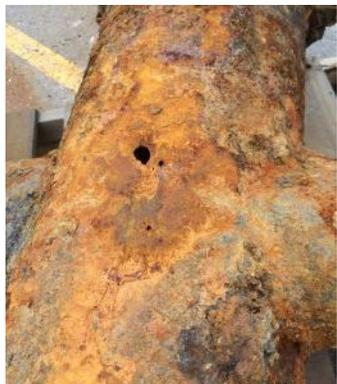
**Figure 5.2-24: Multiple leaks due to severe corrosion on vintage NPS 12 gas main**
