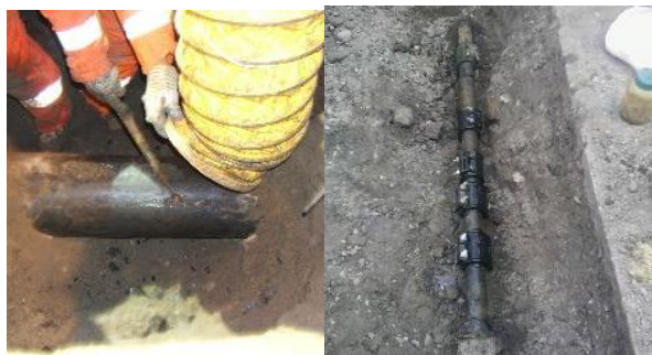
Figure 5.2-7: Bare and unprotected steel failures
