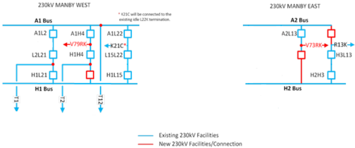
Figure 2:Phase 2 Revised Bus Configuration of Manby East TS and Manby West TS
