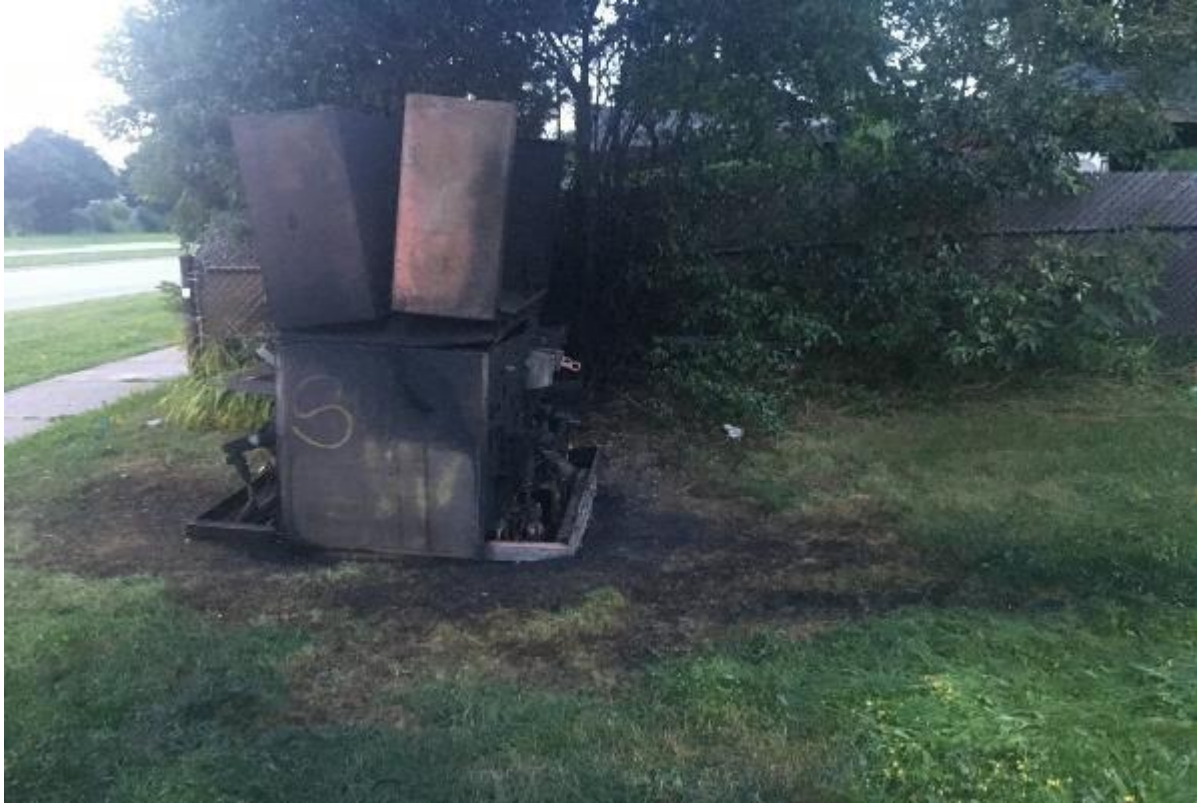
Figure A10 - 15: Failed Oil-Filled Switchgear, August 2018
