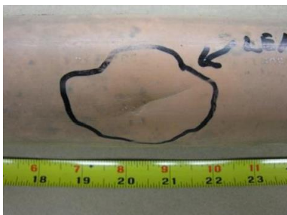
Figure 5.2-59: Sample of Aldyl-A Pipe with Crack Failure
