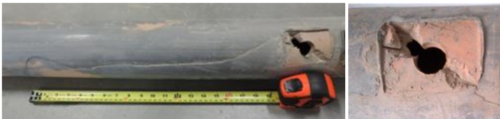
Figure 5.2-35: Rapid Crack Propagation on Aldyl A Pipe from Saddle Tee Fusion (Mississauga, ON)
