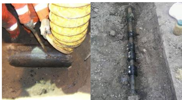
Figure 5.2-7: Bare and unprotected steel failures
