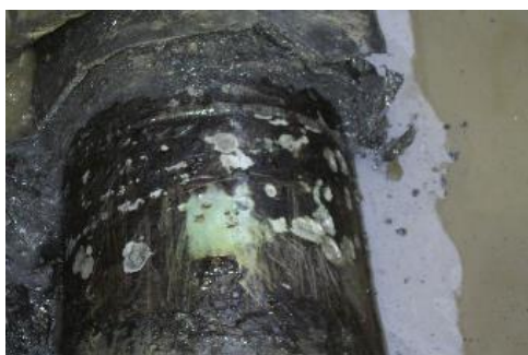
Figure 5.2-52: Multiple corrosion sites on NPS 12 St. Laurent pipe
