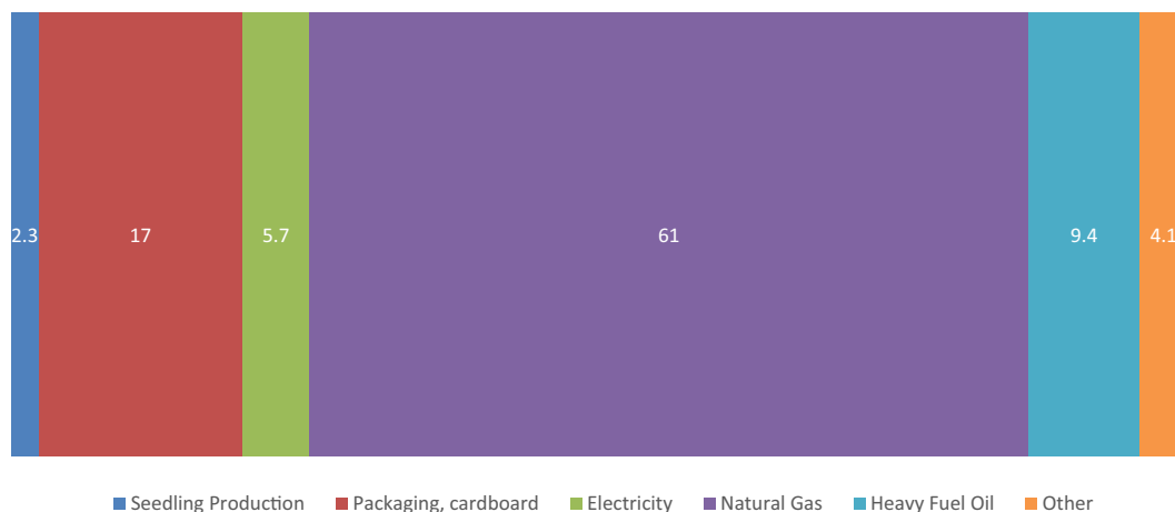
Fig. 3. Cumulative energy demand contribution analysis for producing 1 kg of packaged tomatoes in an average Ontario greenhouse. Numbered labels indicate percentage of total impact. The category of “Other” consists of CED related to infrastructure, fertilizers, plastic packaging, growing media, and pesticides.
