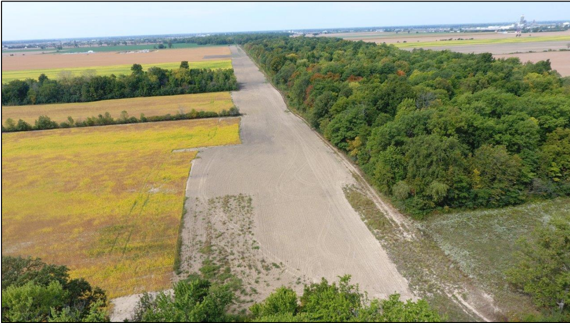
3. An aerial view of the right-of-way after topsoil was replaced and decompaction was completed.
