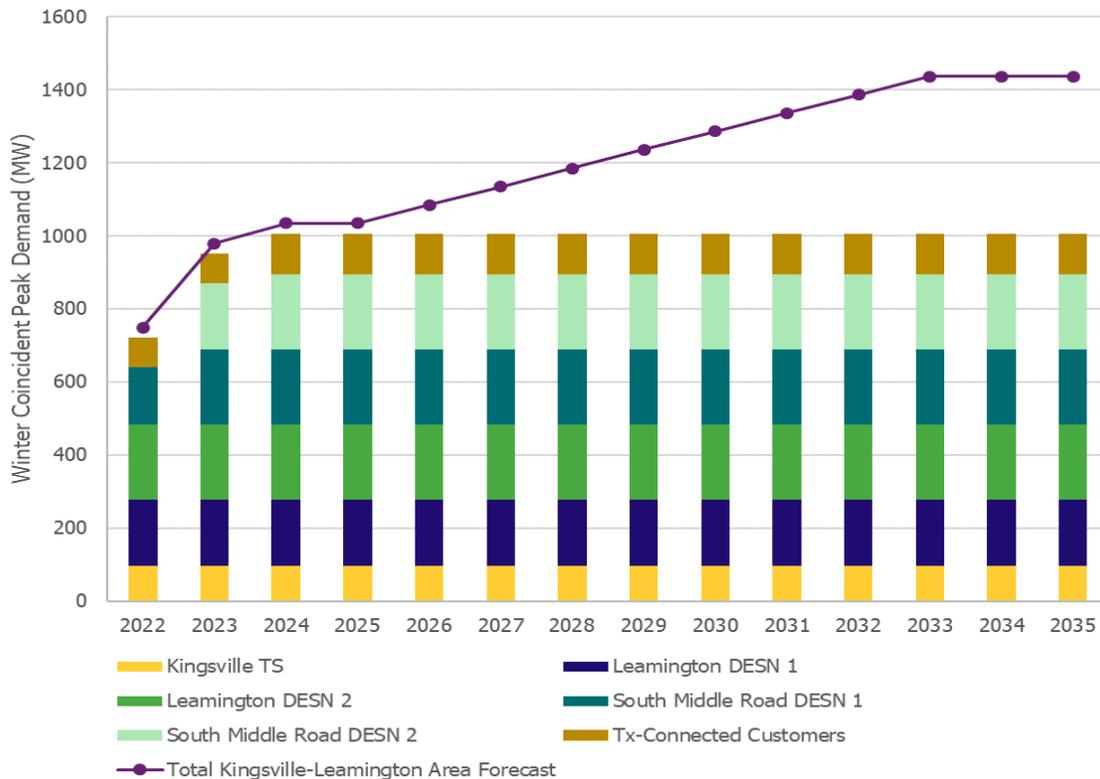
When comparing the capacity that can be allocated to each station against the demand forecast for Kingsville-Leamington (as shown in Figure 5), a local capacity need arises in 2026.<sup>7</sup> This need is expected to be approximately 440 MW by 2035 – of which 410 MW is forecast based on distribution-level greenhouse customers awaiting connection, and the remaining 30 MW is attributed to the already overloaded Kingsville TS.
