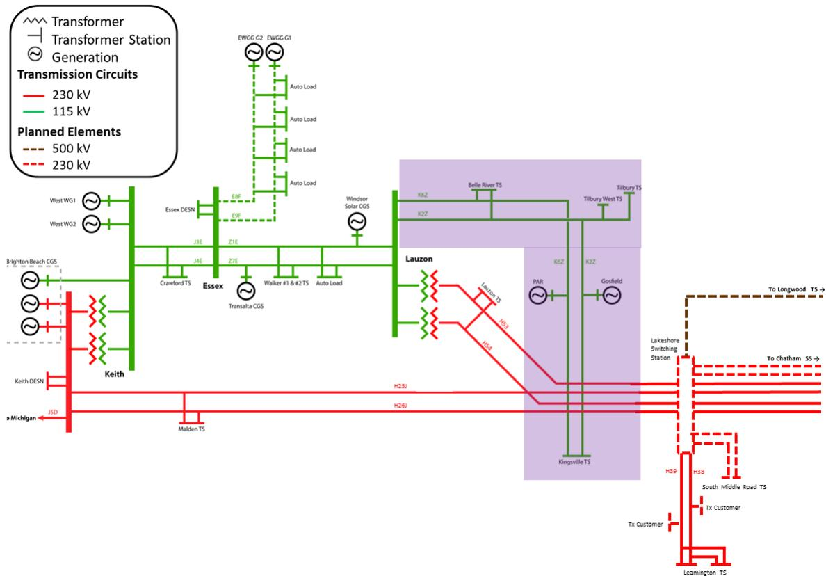
Due to the Lauzon DESN 1 capacity need, the Working Group recommended that T5/T6 be upsized to accommodate the station forecast. Subsequently, since the 2019 IRRP, Hydro One has proceeded with replacement plans for the existing 50/66.6/83.3 MVA two-winding T5/T6 with new 75/100/125 MVA three-winding transformers by December 2025.
