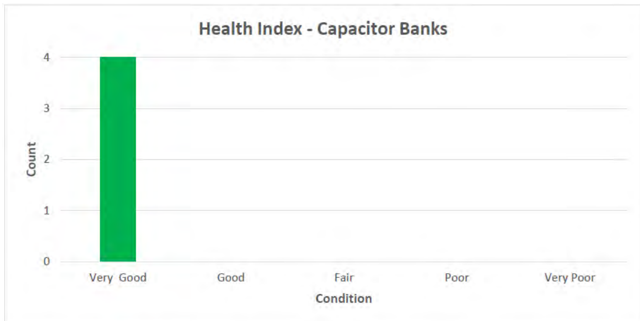
Figure 3.17: Health Index - Capacitor Banks
