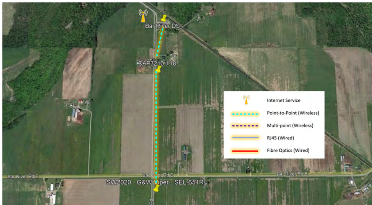
Figure 2: Bar River Hybrid Connection Solution
