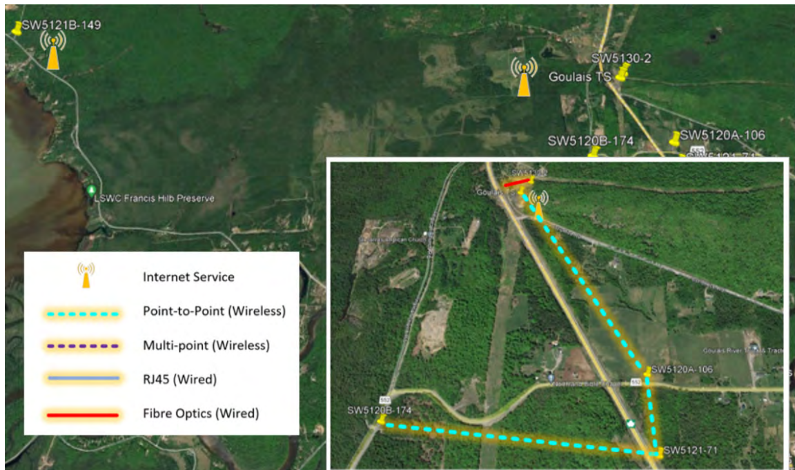
Figure 6: Goulais Hybrid Connection Solution
