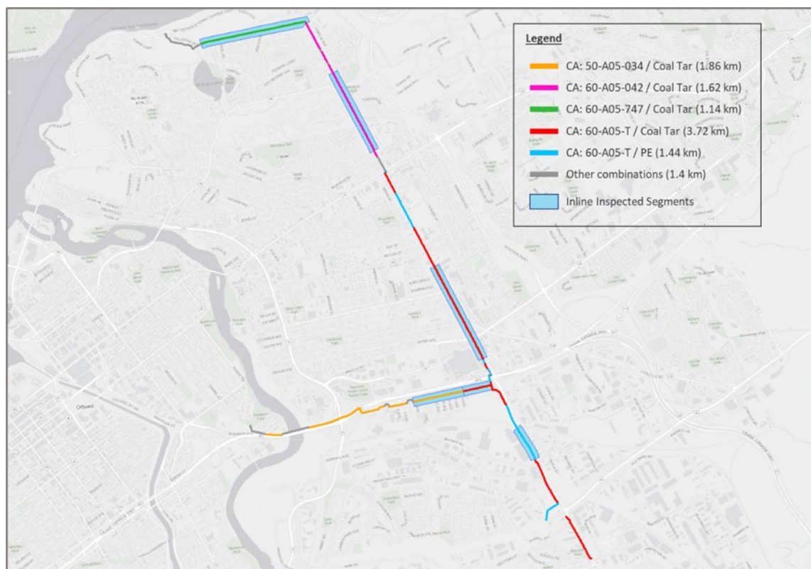
Figure 4: Pipeline Groupings with ILI Locations
