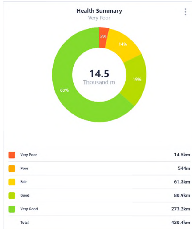
Figure 5.3-14: Overhead Conductor HI Results
