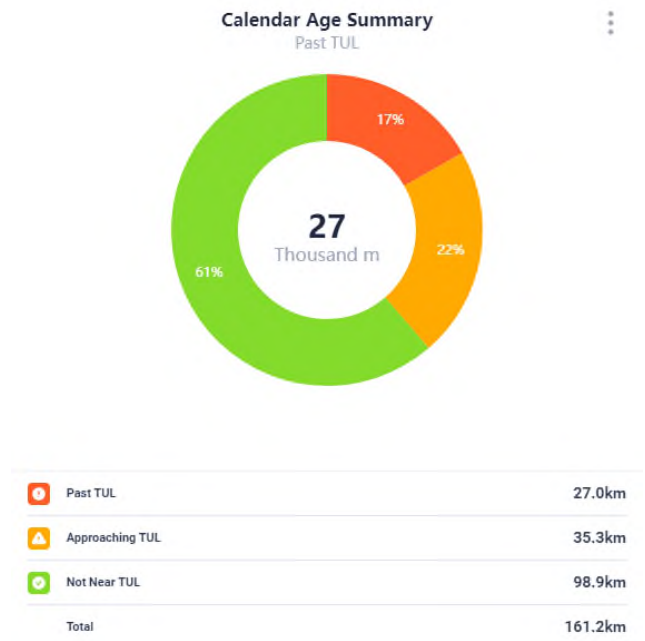
Figure 5.3-17: Underground Cable Age Demographic Summary
