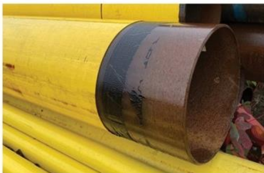
Typical steel pipeline with protective coating
