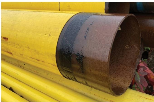
Typical steel pipeline with protective coating
