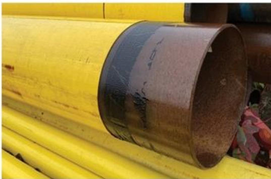
Typical steel pipeline with protective coating
