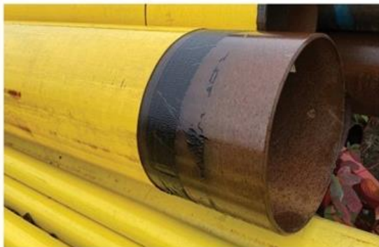
Typical steel pipeline with protective coating
