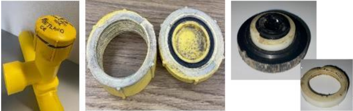
Figure 6.2-38: Examples of Cracked Caps
