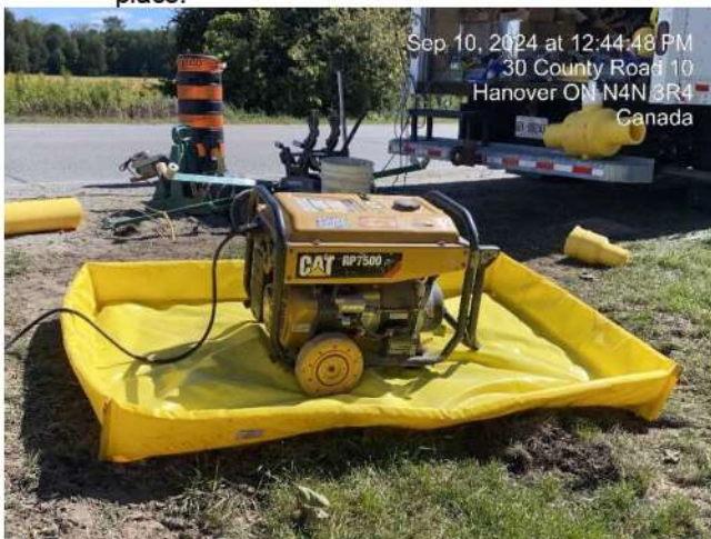
Photo 5 Secondary spill containment around potential source of contamination.
