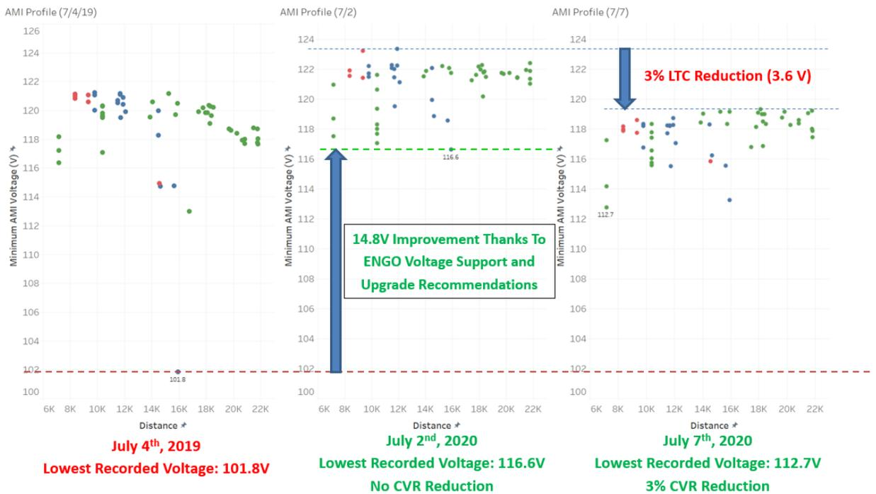
Figure 23: X07487 Transformer Replacement and ENGO ON (May-July 2020)
