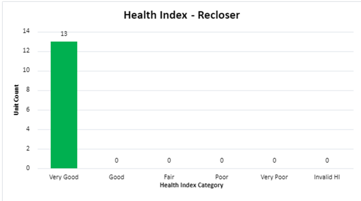
Figure 4-26: Overhead Line Recloser HI Results
