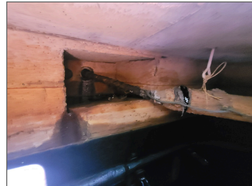
(b) Underground cable failure
