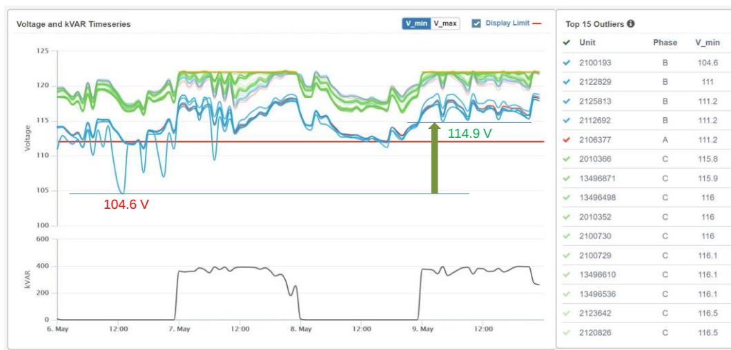
Figure 11: GEMS plot shows voltage improvement as a result of the transformer upgrade and ENGO devices deployed in the field from an initial low voltage of 104.6V to a final minimum voltage of 114.9V
