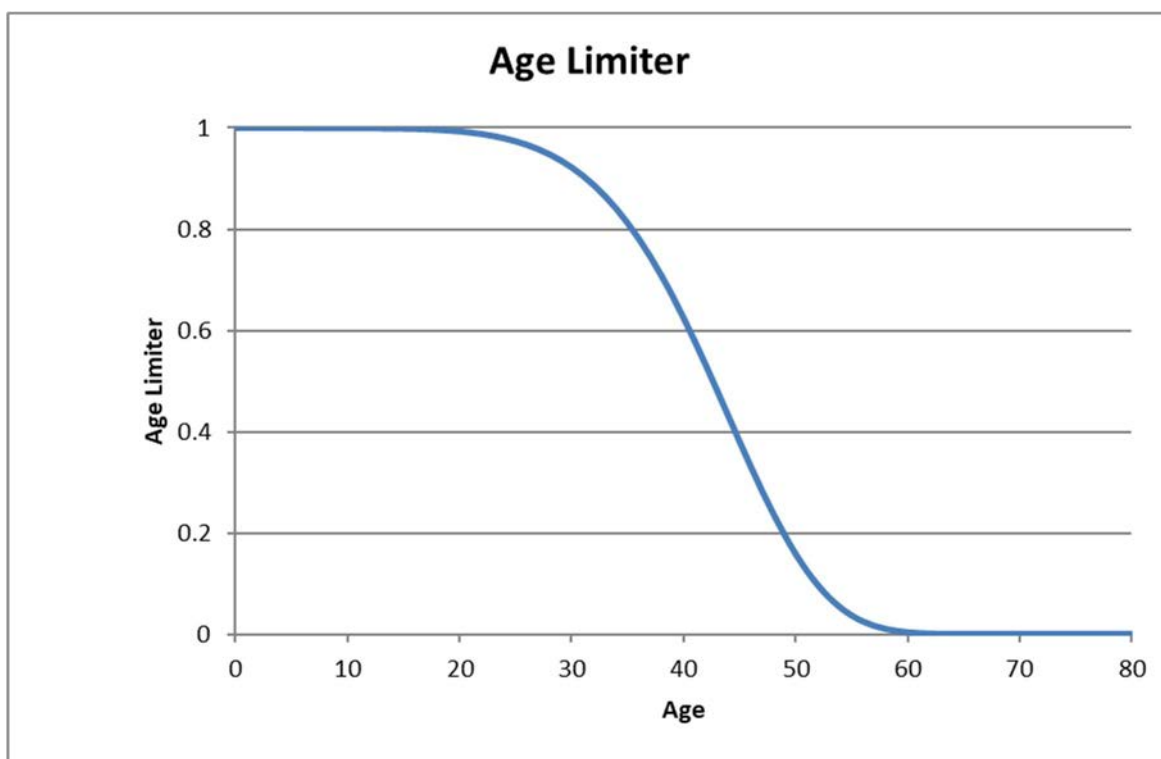
Figure A 1-2 Power Transformers Age Limiter
