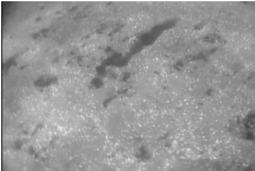
Figure 3.1 - Video still frame images of the surficial sediments present within Unit A. The images show soft clay sediments with abundant shell fragments and shell beds. Algae is also present on the lake floor, visible in the bottom two images.
