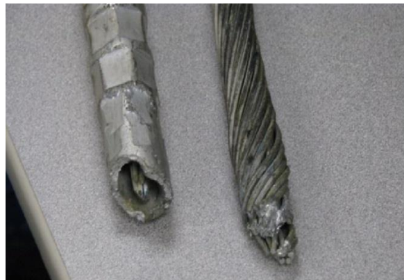
Figure 2 - Broken ACSR Conductor
