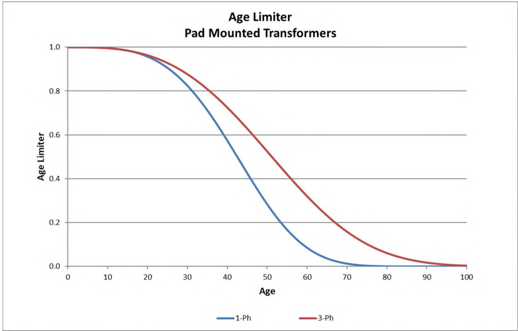
Figure 2-1 Age Limiting Factor Criteria - - Pad Mounted Transformers
